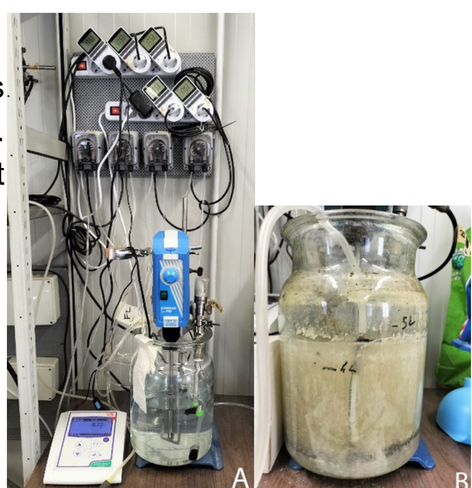
SBR reactor setup: stirrer, Do probe, ph meter, peristaltic pumps, aeration and timed sockets.
