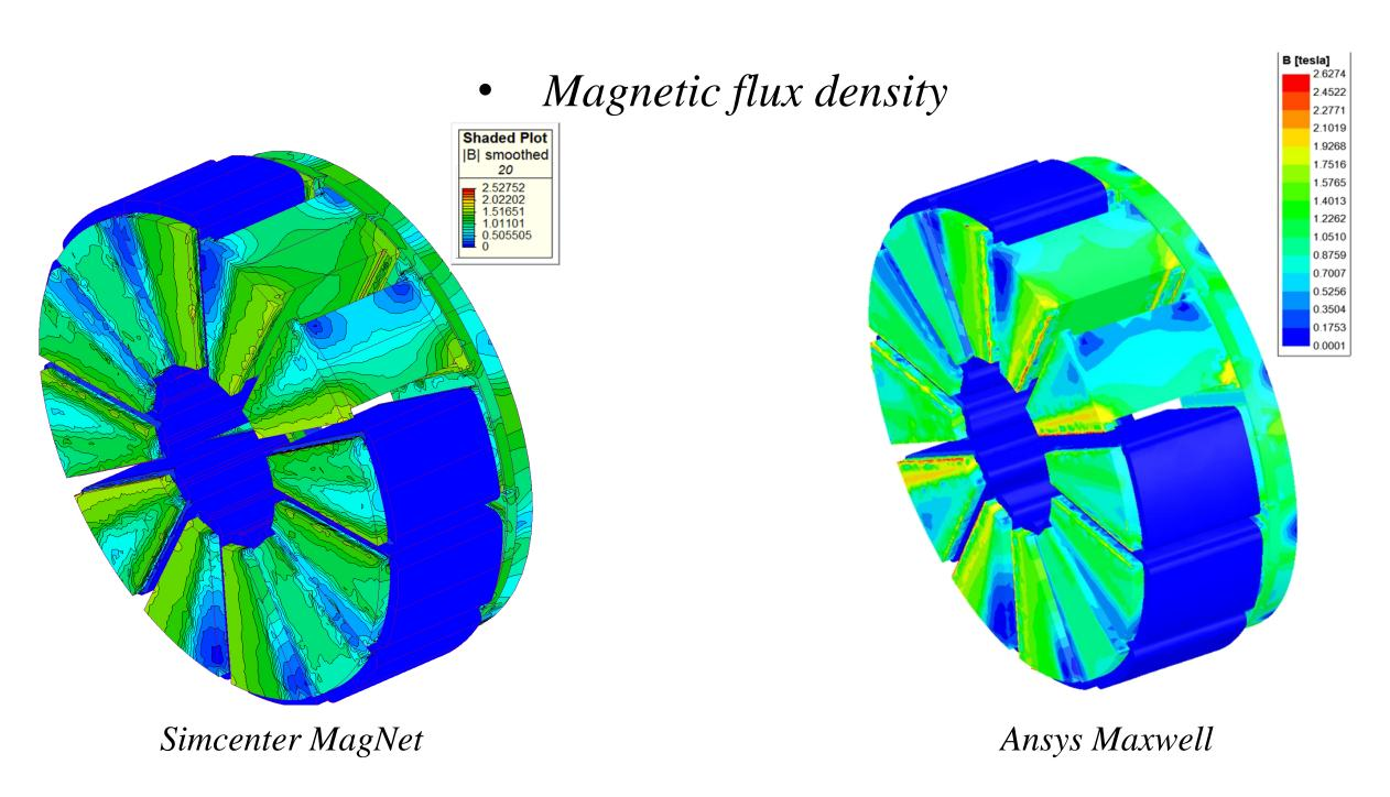
The maximum of the magnetic flux density is in the fitting radius that links the head and the body of a tooth.
