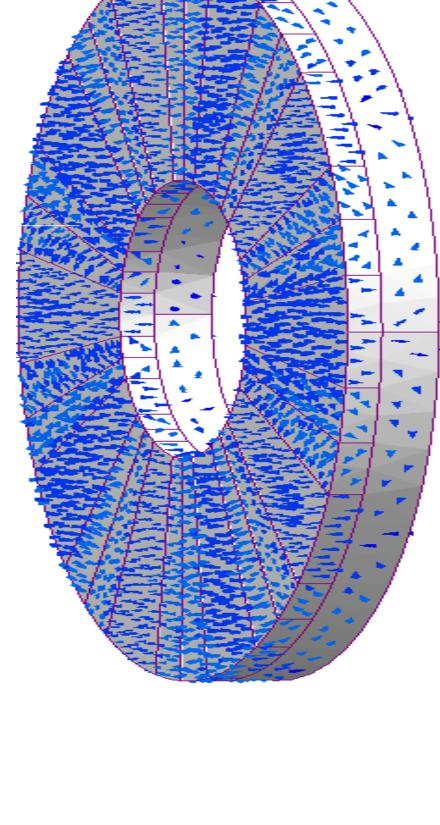
The rotor position for which we have the maximum torque does not change, but its value grows more than 10 %.
