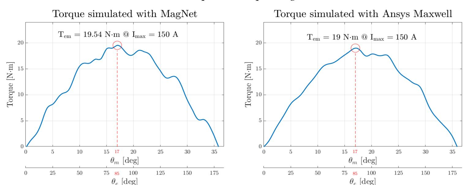
The developed torque depends on the angle between the spatial vector of stator currents and the vector representing the magnetic flux produced by permanent magnets (i.e. the torque angle). When the two vectors are perpendicular, electrically speaking, the device develops the maximum torque. Due to some torque oscillations this does not appear from simulation results.
