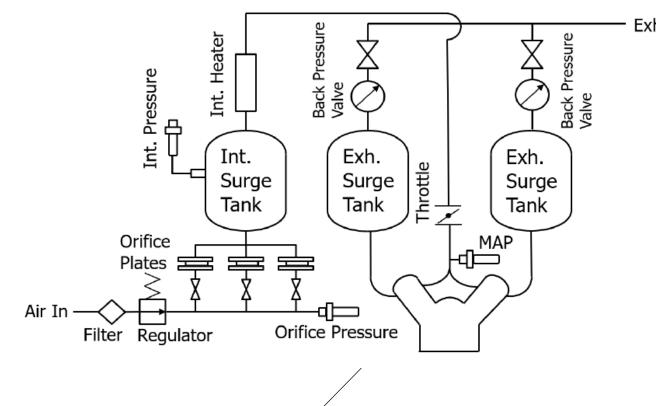
A particular air supply system allows to take data while the engine is breathing at constant intake pressure and temperature, and between a constant pressure drop, to ensure that the ambient variables do not influence on the operating conditions.
