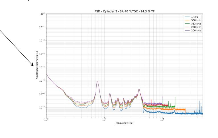
During the experimentation, knocking conditions were induced by acting on the spark ignition advance values in both cylinders.
